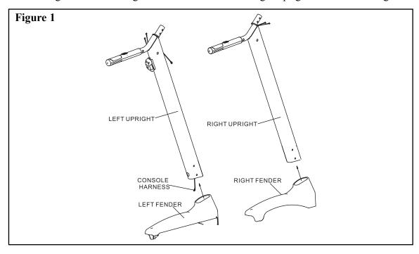
2. Slide the fenders up the upright assembly and pull the console harness through the hole in bottom of the left upright tube as shown in Figure 2.
